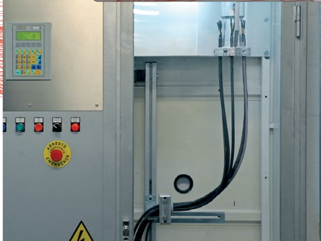
TORSION TESTS \pm 360^\circ WITH ADJUSTABLE ACCELERATION RATE
