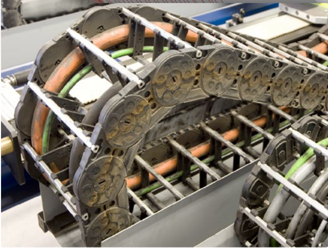
DYNAMIC TESTS ON CHAIN TRACKS UP TO 17 METERS
